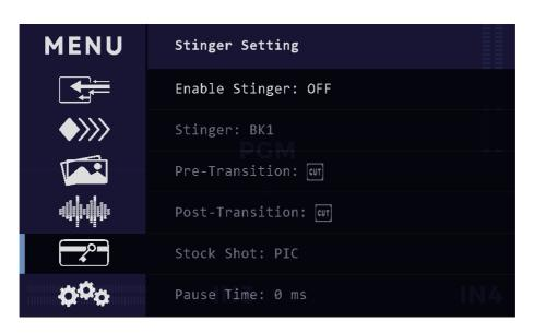
In the process of stinger effects, use the one-way method when using AUTO transition, and use the two-way method when using T-BAR transition.
